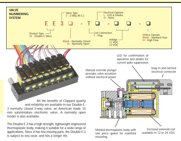
Double E-3 Valves are available factory assembled on manifolds
